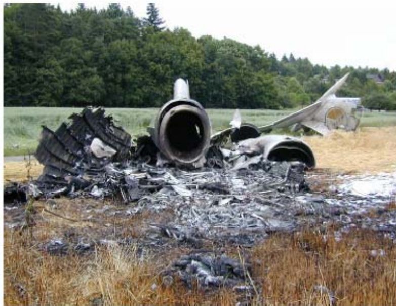
overall view – rear fuselage section/tail unit
