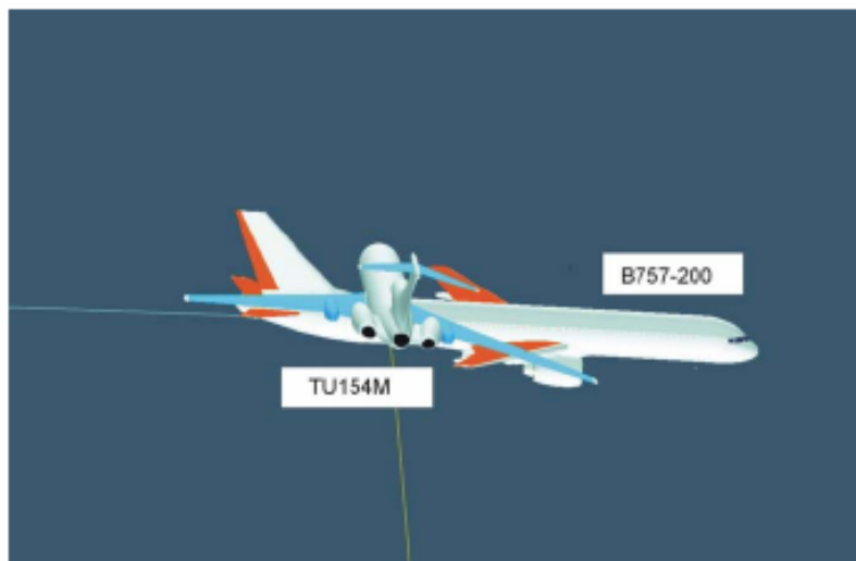
Reconstruction of the collision according to FDR data and collision evidence
